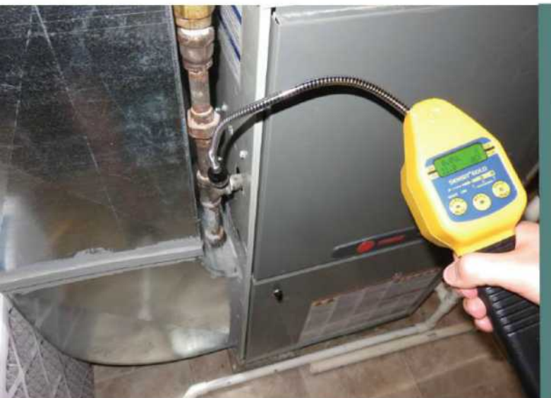
Intrinsically safe gas leak detector
