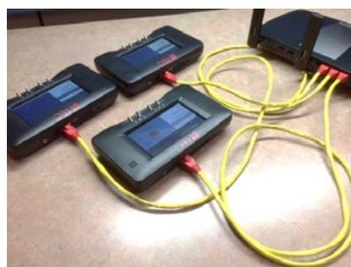
4. Plug in one end of the Ethernet cord into the DG-1000 Ethernet port and the other end into the Ethernet port on a router or switch.
