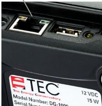
The Ethernet port on the DG-1000 can be used to create a network of gauges that can be used for specialized testing applications, such as big building airtightness testing. Using the gauge's Ethernet port to create a wired multi-gauge network requires a router. A standard
