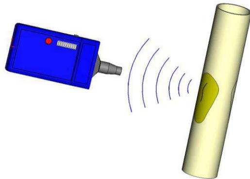
The intensity of sound generated at a leak is a very complex function of the viscosity, the temperature, the speed the fluid is moving, the Reynolds number, the pressure differential across the leak, and the physical dimensions and characteristics of the orifice. This is why it is possible for a **smaller** leak to generate **more sound** than a larger one.
