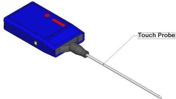
Being careful not to cross the threads, simply unscrew the existing nose piece and replace with metal probe. Place the tip of the probe on the item being tested with just enough force to hold it in place. Be careful around moving equipment.
