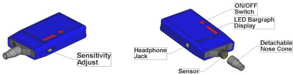
The **AccuTrak<sup>®</sup>** VPE is capable of hearing leaks from over forty feet away, but it is best to hold the instrument as close to the test area as safely possible. Check around fittings and piping using a zigzag motion, carefully covering all suspected areas. If there is no ultrasonic sound present, the display should not have any lights on. When an ultrasonic signal generated from a leak is
