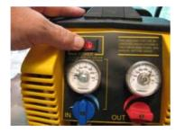
After opening both valves and turning the machine on, close the output valve and wait until the pressure reaches approximately 550psi and trips the high pressure switch (which should take less than a minute).
