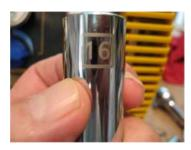
Probably the easiest way to remove the input and output fittings is with a a 5/8" (or16mm) deep well socket, keeping track which is the inlet and outlet fittings.
