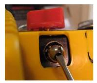
Again, use a small screwdriver to align the ball valve in position. Also remember to seat the handle it points towards the gauge.
