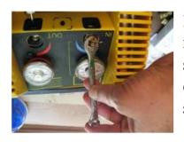
Insert the valve stems and tighten. Look into the input/output ports and turn the stems until the tabs are inline with port opening and will allow the ball valve to slide in freely.
