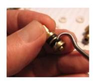
Carefully replace the two smaller O rings; this can be a bit tricky!
