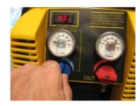
Turn the switch off (to prevent starting again when the pressure drops) and quickly close the inlet valve attempting to keep approximately 400psi of pressure in the machine. Once the input valve is closed, the pressures should equalize.
