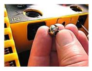
ball valve to make certain it is replaced properly. There are three holes in the ball, two large and one small with a groove the valve stem fits in. The smaller hole points to the left when reinstalled.
