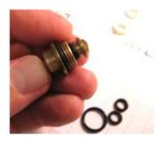
Each valve stem has 3 O rings; two small and one large. Push the core out of the housing to access the smaller O rings. Use a pick or small needle nose pliers to remove the old O rings.
