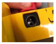
Again, align the tab on the input valve stem to allow the ball valve to slide in and position the red knob so it is pointing directly at the gauge.
