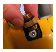
Remember, you are trying to shape the Teflon seals against the ball. Seating the fittings with the valves open, may damage the seals.
