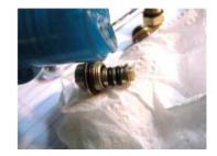
Replace the O rings on the inlet and outlet port fittings.
