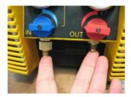
A quick field test can also be done by putting your fingers over the ports and see if you can feel pressure leaking out.
