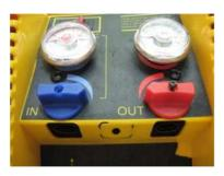
Remove the screws from the red and blue input and output knobs and set aside.
