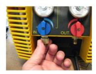
This is done by removing any refrigerant hoses *and checking the input screen to make sure it is clean*.
