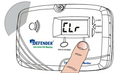
Each reading will appear for five seconds. To erase the record in memory, press the Display Memory button, and while the readings are being displayed, press the **TEST/RESET/MUTE** button. The monitor will burst a long beep, and the display reads
