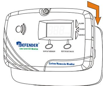
Connection between mounting plate and monitor will turn activation switch **ON**.
