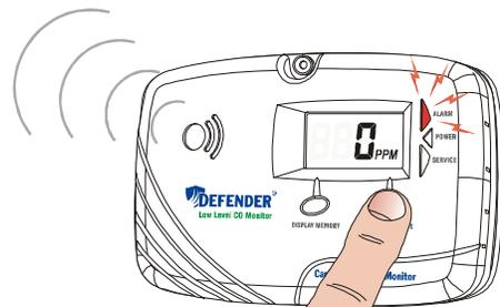
**LCD DISPLAY FUNCTION:** When monitor is operating normally, the LCD will display 0 PPM or the current CO level if 5 PPM or more is detected. Above 500 PPM, the LCD will flash "500 PPM". The LCD will display
