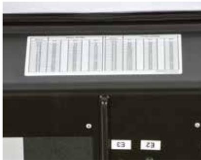
If you are not using one of our pressure gauges, the pressure reading taken from the metering box can easily be converted to air flow using a flow table attached to the side of the metering box.
