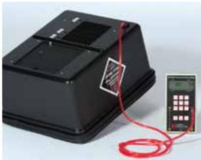
The lightweight Exhaust Fan Flow Meter makes easy work of low flow airflow measurements.
