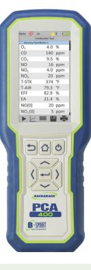
The MSA Bacharach® PCA® 400 is a handheld versatile combustion and emissions analyzer for commercial and individual applications. The analyzer may be configured for up to 4 gas sensors, including  $O_2$ , CO, NO, NO<sub>2</sub> and SO<sub>2</sub>. The PCA® 400's portable and durable design is ideal for testing, tuning, and maintaining burners, engines, furnaces and variety of other commercial and industrial combustion applications.
