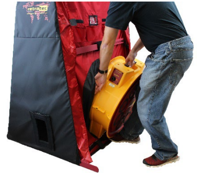
Figure 11: Installing a fan in the cloth door panel.
