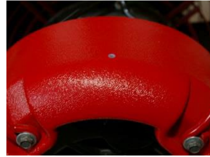
Figure 17: Pressure sensor on the fan motor casing.
