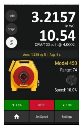
Picture of DM32 display showing Leakage Factor of 10.54 CFM/100 sq ft @ 4.0000 in WC on Channel B.
