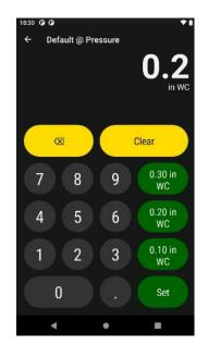
Since you must not exceed the test pressure, the actual pressure will be lower but entering this default will ensure that all flow results are displayed as a value extrapolated to the exact test pressure entered.
