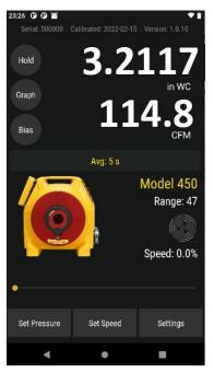
Picture of DM32 display showing Leakage of 114.8 CFM @ 4.0000 in WC on Channel B.
