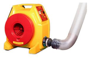
A Flow Conditioner is not needed with Retrotec fans for depressurization testing. Some duct testing fans require a flow conditioner when depressurizing a duct system, in order to get correct readings. The Retrotec DucTester does not require a flow conditioner because it uses a flow nozzle, which is intrinsically stable in either direction because the flow gets compressed as it goes through the nozzle.
