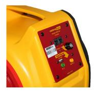
Figure 1: Retrotec Model 400 has a speed control knob and two Ethernet style Speed Control Ports for daisy chaining speed controls for running many fans together. The yellow and green color coded tubing connections to the gauge are shown.
