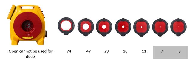
Figure 5: Range 74 is for the leakiest ducts while the smaller ranges are for progressively tighter ducts.
