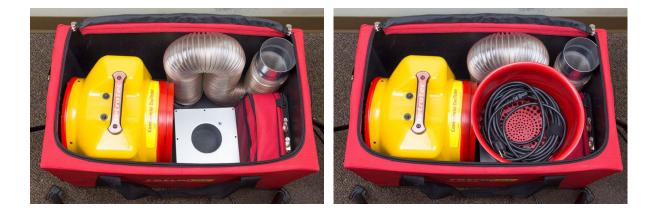
Model 450 above is a tight fit and needs to be packed in exactly the correct order, or the components will not fit.
