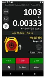
In the example on the left, the Device is set to "450" and Range to "47". It is very important to ensure these are both correct. The Range is engraved in the orifice plate which also has a raised color sticker which is printed with "Range 47" in the case of this example.
