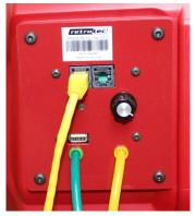
To test control of the fan, press **[Set Speed] [1] [Set]** on the gauge. This sets the fan to 1% speed on the gauge but achieves about 15% speed on the blower.
