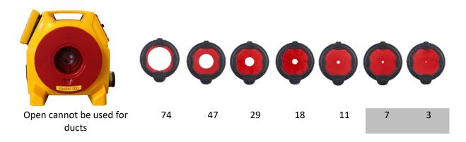
Figure 6: Range 74 is for the leakiest ducts while the smaller ranges are for progressively tighter ducts.
