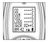
CO/CO2 displays CO (ppm), Losses calculated, Excess air %. Make any adjustments needed for proper Combustion and wait for analyzer to display change in readings. (Repeat as necessary).
