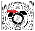
Rotate function rotary dial to TEMP for Temperature Test Screen
