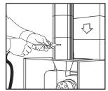
Remove the probe from the flue and allow analyzer to purge with fresh air until readings return to zero. 02 to 20.9%, CO to Zero **CAUTION:** probe tip will be HOT.
