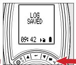
To Log: During testing, Press and Hold to log a report.
