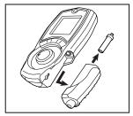
Remove protective rubber boot. Remove water trap from analyzer. Remove particle filter from spigot and replace with new one. Reattach trap and boot.
