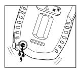
Remove the rubber boot and red drain plug. Allow the water to drain out. Re-insert the rubber plug and replace boot cover.
