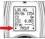
To print the LOG, Press ▲ and ▼ buttons until PRINT is selected between two arrow icons. Press ← to select to start printing.
