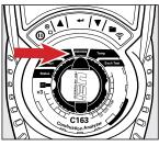
Rotate the function rotary dial to CO/CO2 for Test Screen 2 parameters.
