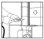
Remove the probe from the flue and allow analyzer to purge with fresh air until readings return to zero. O2 to 20.9% and CO below 20 ppm
