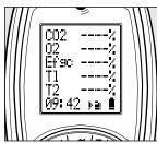
02/Eff displays C02, 02, Efficiency, Flue temperature, Inlet temperature.
