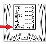
Press ▼ button until the Fuel Type displays on the Status Bar. Press and Hold ← until two arrow icons display.
