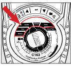
Rotate the dial to either STATUS, AUX, 02/Eff, C0/C02 or Temp setting.
