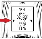
Rotate the dial to MENU. Press button until the LOGS is selected between two arrow icons. Press to select.
