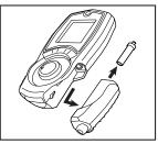
Remove protective rubber boot. Remove water trap from analyzer. Remove particle filter from water trap and replace with new one. Reattach trap and boot.
