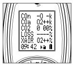
CO/CO2 displays CO (ppm), CO2, Losses calculated, Excess air %. Make any adjustments needed for proper Combustion and wait for analyzer to display change in readings. (Repeat as necessary).
