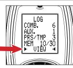
Screen displays all saved LOGS. With VIEW selected in the Status Bar, Press 🗲 to select.
