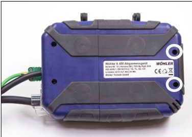
Fig. 48: Bottom of the device - Open the cover by loosening the cross-head screws .
