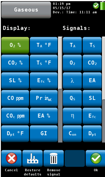
Fig. 36: Configuration of the readings segment.
