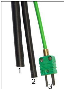
Fig. 16: Gas probe – gas hose (1), pressure hose (2), temperature plug (3)
